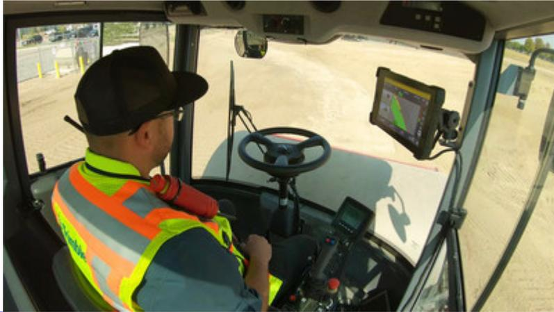
Trimble Earthwork's Horizontal Steering Control automatically steers a soil compactor using a 3D model or compaction pass line. This helps to improve compaction productivity and quality for operators of all skill levels by precisely controlling overlap between passes. Auto steering helps reduce operator fatigue while also minimizing over- and under-compaction, providing a more consistent sub surface for a higher quality, longer lasting finished product.
