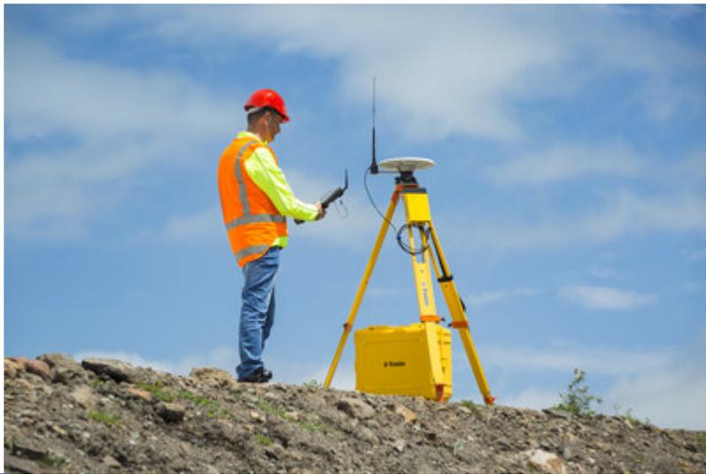
The R750 can be used to broadcast Real-Time Kinematic (RTK) corrections for a wide range of applications, including seismic surveying, monitoring, civil construction, precision agriculture and more. Access to all available satellite signals provides improved performance and reliability when used with a Trimble ProPoint™ Global Navigation Satellite System (GNSS) rover. ProPoint gives users improved performance in challenging GNSS conditions, with ground-breaking signal management.
