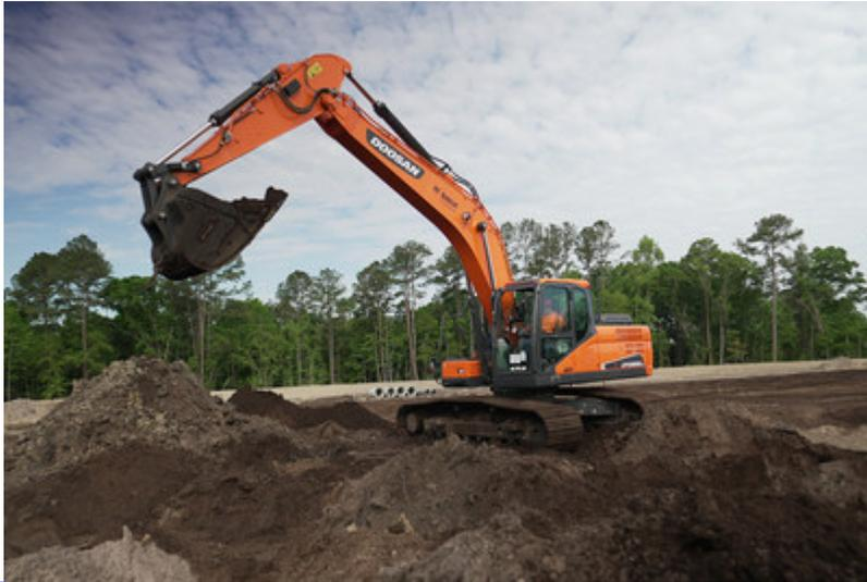
Doosan will offer a 2D machine control factory-installed option that includes a 10-inch Android™ tablet display running the Trimble Earthworks software application. This option includes rugged Trimble hardware, designed and tested for the harsh conditions found on construction sites.
