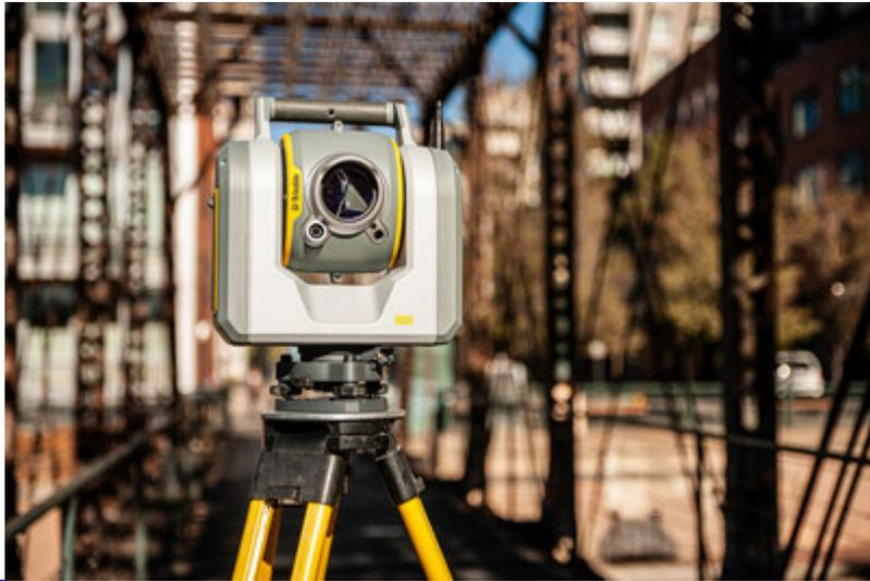
The Trimble SX12 merges high-speed 3D laser scanning, Trimble VISION™ imaging technology and high-accuracy total station measurements into familiar field and office workflows for surveyors. A new green, focusable Class 1M laser pointer is safe for viewing with the naked eye, offers high-power visibility and makes it easy to see even at a distance. An improved camera system provides enhanced pointing and site documentation capabilities.
